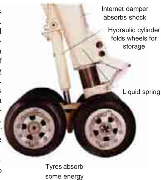
**Landing Gear :** When an aircraft comes in to land, it has to lose a lot of energy in a very short time. the landing gear deals with this and prevents disaster. First, mechanical or liquid springs absorb energy rapidly by being compressed. As the springs relax, this energy will be released again, but in a slow controlled manner in a damper-the second energy absorber. Finally, the tyres absorb energy, getting hot in the process.
