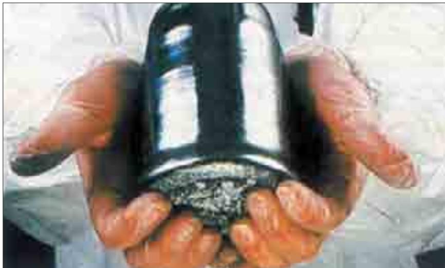
**Gallium arsenide (GaAs)** is now being manufactured as an alternative to silicon for microchips. This combination of elements is a semiconductor like silicon, but is electronically faster and therefore better for microprocessors.
